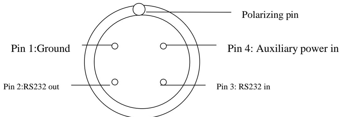
Figure 1: Connector on end of cable – supplied optionally.
