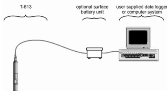
It is operational to a depth of 100 meters. Optional Yeo-kalSoft software makes it a complete Water Quality Analyser, with data logging onto the computer and graphical analysis and display.
