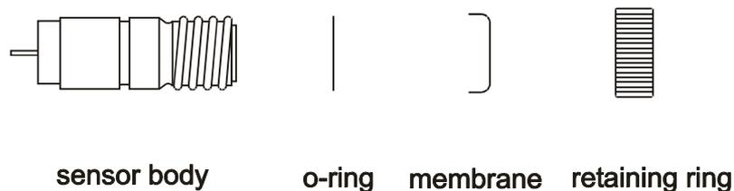
Figure 4: Exploded view of dissolved oxygen sensor.
